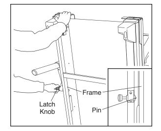
2. Hold the metal frame firmly with both hands and lower it to the floor. CAUTION: Do not grip only the plastic foot rails or drop the frame to the floor. Bend your legs and keep your back straight.
